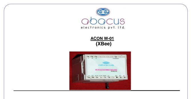
**INTRODUCTION:** - The ACON W-01 is serial to wireless converter .The XBee modules operate within the ZigBee protocol and support the unique needs of low-cost, low-power wireless sensor networks. The XBee module interface to a host device through a logic level asynchronous serial port. Through its serial port, the module can communicate with any logic and voltage compatible UART; or through a level translator to any serial device . The modules operate within the ISM 2.4 GHz frequency band.
